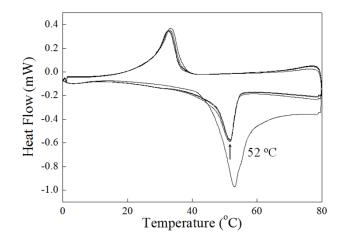
Fig. S6 DSC data of PA-PDA ( $C_{23}$ -GAGAGAGY), with heating and cooling rate 10 K/s. The repeated endothermic peaks appeared at 52 °C.
