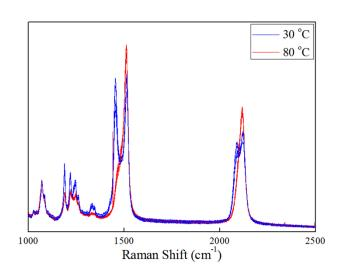
Fig. S3 Raman spectra of PA-PDA membrane at temperatures 30 °C and 80 °C, red 6 times, blue 6 times.
