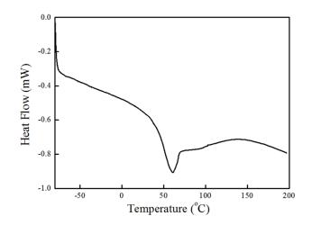
Fig. S5 DSC data of PA-PDA (C<sub>25</sub>-GAGAGAGY) at temperature from -80 °C to 200 °C. Only one peak (excluding water peak) at 60 °C appeared.
