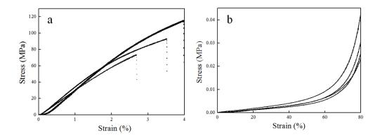
**Fig. S1** Mechanical properties of PA-PDA fibres (a, tensile test, tensile modulus 3 GPa) and gels (b, compression test, compression modulus 10 kPa). Different curves in a) and b) mean multiple measurements.
