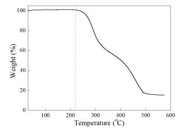
Fig. S4 Thermogravimetry analysis (TGA) of PA-PDA materials, indicating no thermal degradation below 200 °C.
