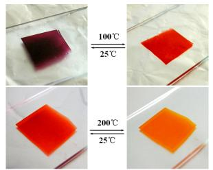
Fig. S2 Color transition between temperatures 25 - 100 °C and 25 - 200 °C. The materials still have obvious reversibility even heated to 200 °C.
